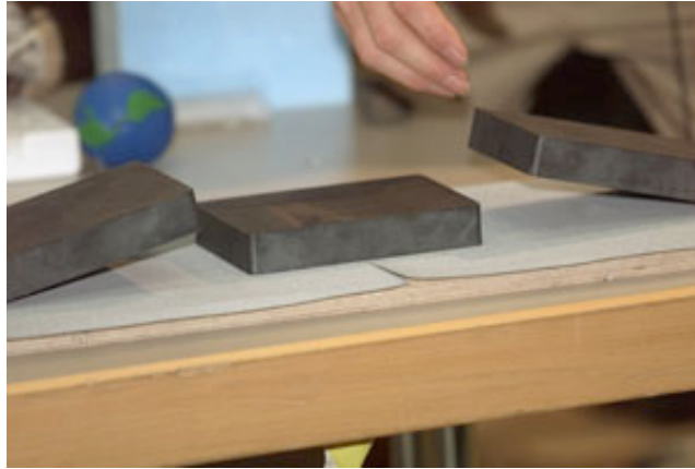
Magnetic oscillators made with large slab magnets.
